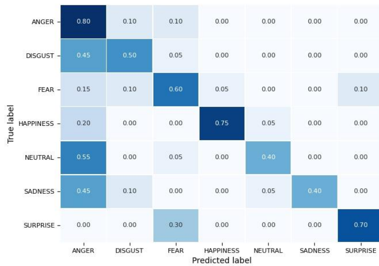
Figure 25 – Confusion matrix of the VGG16 model for the Net Images dataset.
