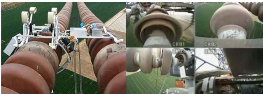
Figure 2.1: Insulator inspection using a climbing robot, with examples of the data provided by it (Source: [4]).
