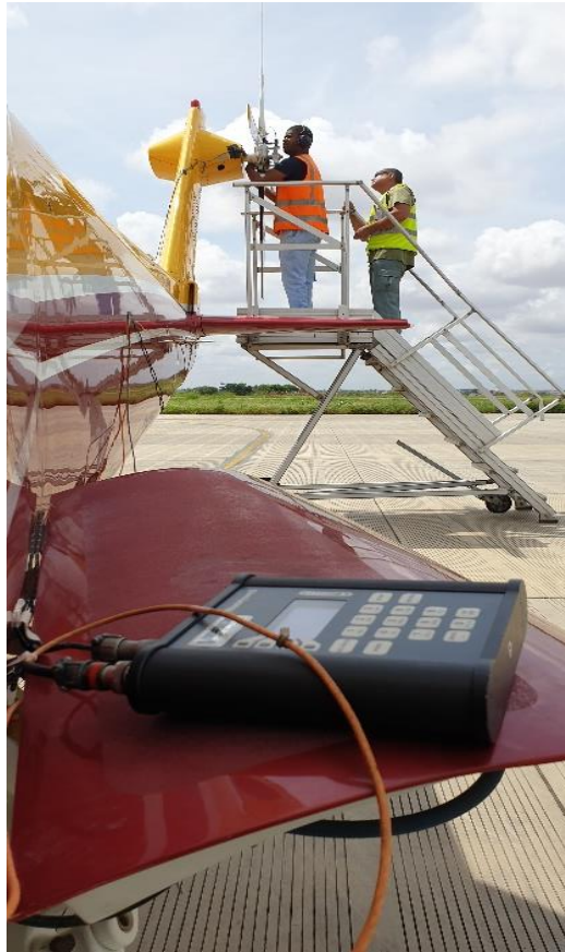
Figure 4: Balance of the tail rotor blades with digital signal processing techniques. Source: Photograph taken by the author on the 01/03/2019 at FNLU of Maintenance Technician Flávio Silva and Maintenance Senior Avionics Specialist Elvis Alves
