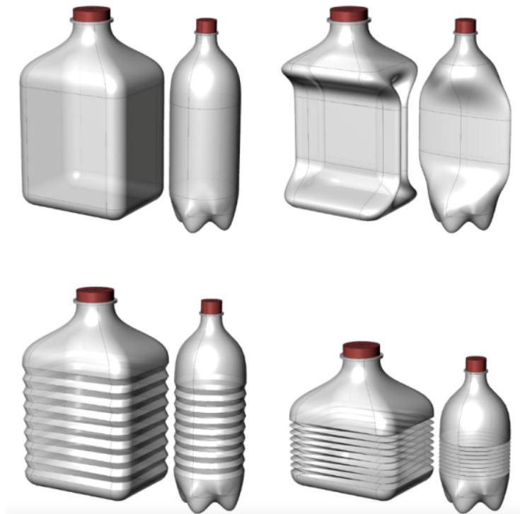
Figure 15. Current bellows systems ineffective collapse and damage the package (Source: WisePack archive, 2008)
