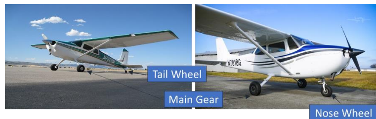
Figure 28. Conventional landing gear (left) and tricycle gear (right)
