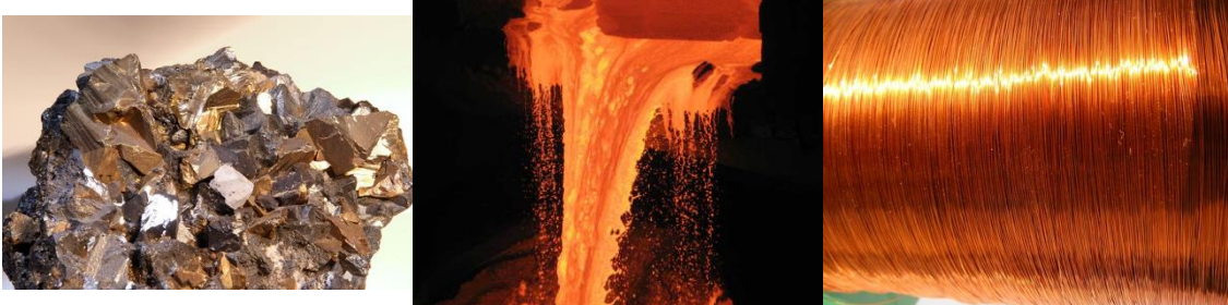
Figure 8. From copper ore to copper wire: (a) chalcopyrite ( \text{CuFeS}_2 , with 34.5 % copper) is one of the several copper ores; (b) it can be refined into copper metal by smelting; (c) and then the metal is formed to the final desired product shape.
