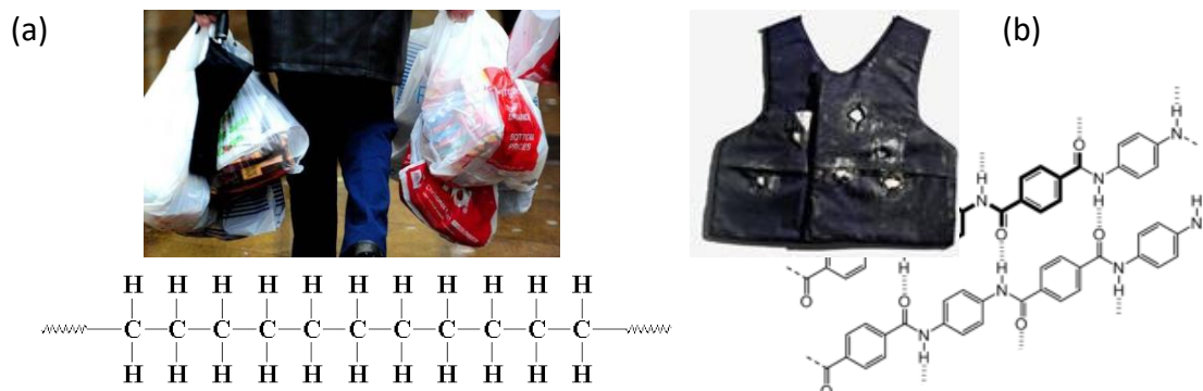
Figure 11. Polymer diversity, from (a) polyethylene application in grocery bags, to (b) Kevlar® vest after shot. The corresponding molecular chains are shown at the bottom of each image.
