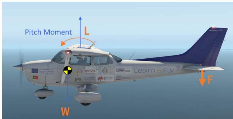
Figure 68. Principal Vertical forces acting in and aircraft.
