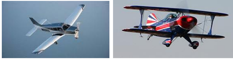
Figure 24. Monoplane (left) and Biplane (right)
