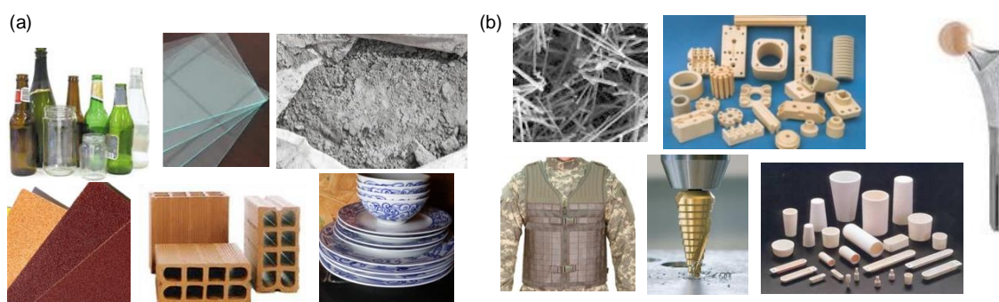
Figure 10. Some examples of application of ceramic materials. (a) Traditional ceramics (clock-wise): glass bottles, plain glass, cement, porcelain, brick, abrasives. (b) Technical ceramics (clock-wise): reinforcement fibres, electric insulators, bioceramic coating on hip prosthesis, lab material, hard coating on cutting tool, tiles in ceramic armour.
