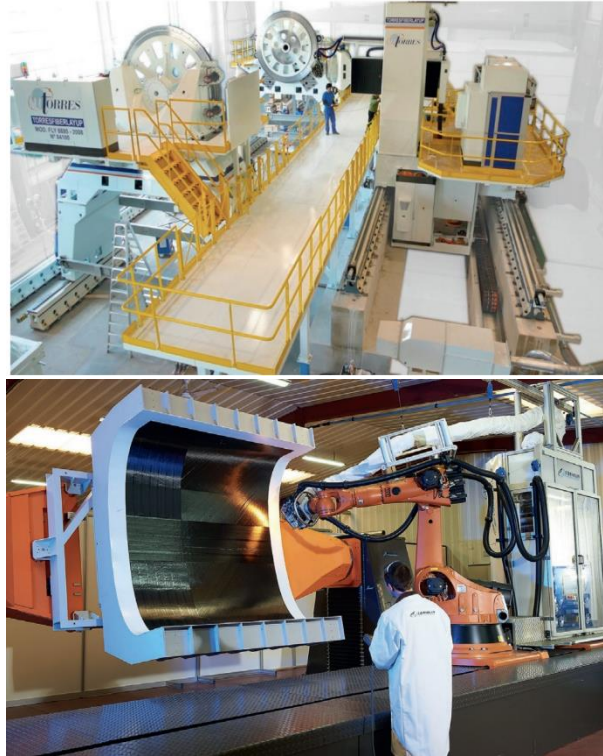
Figure 52. Automated fibre placement [35]: (a) example of commercial equipment (MTorres Machine Company, Spain); (b) Robotic AFP in several orientations (Coriolis Composites, France).
