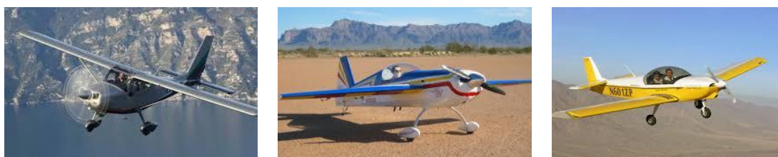
Figure 23. High-wing (left), mid-wing (center) and low-wing (right)
