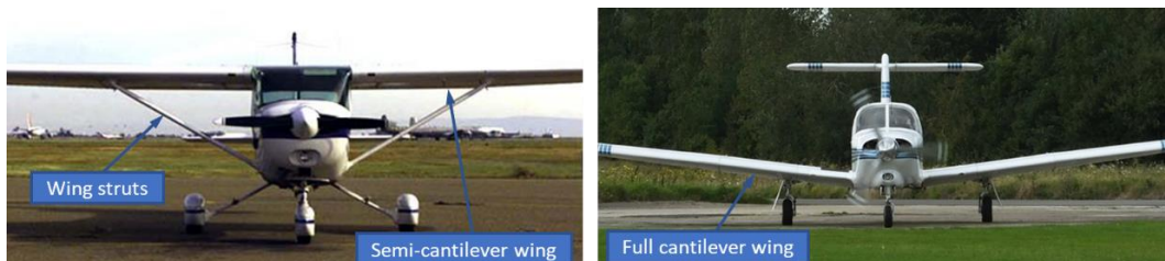
Figure 25. Semi-cantilever wing (left) and full cantilever wing (right)
