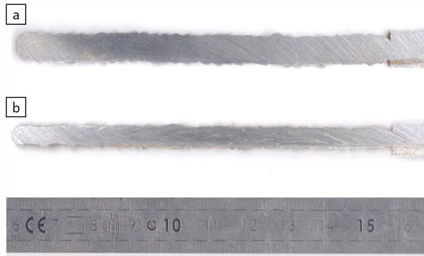
Figure 4.1 – a) High heat and b) low heat-input cross sections.
