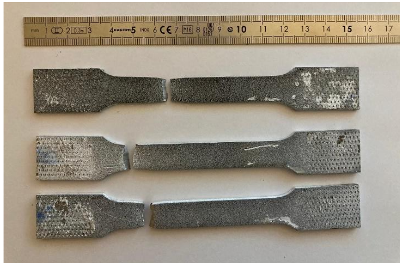
Figure 4.14 – Fracture location after testing on a) 3L and b) 4H (VIC) specimens.
