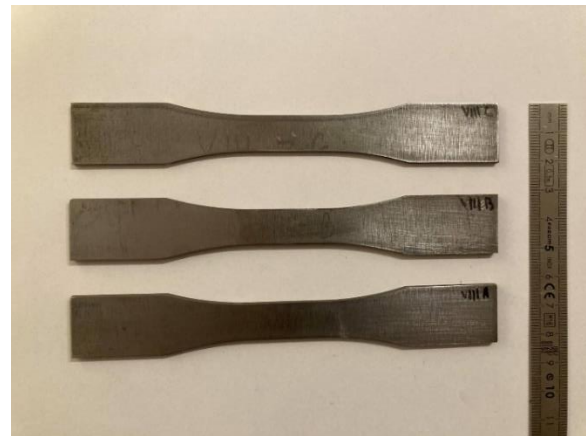
Figure A.1 – Tensile and fatigue specimens produced by EDM.
