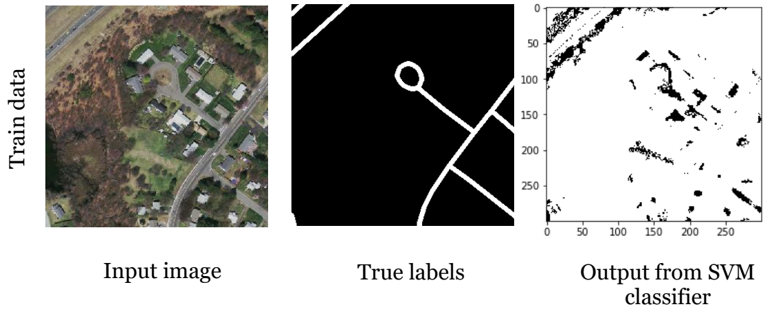
Figure 5.5: A sample input image its corresponding image labels and output from support vector machine classifier for train data set
