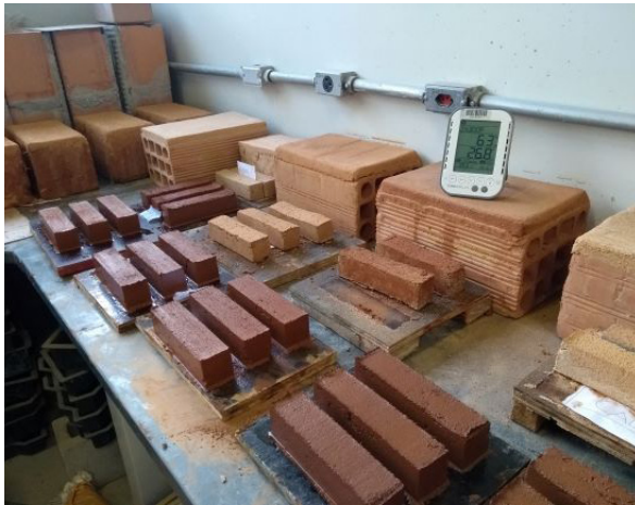
03 Prismatic samples and plaster samples on adobe and brick in the laboratory
