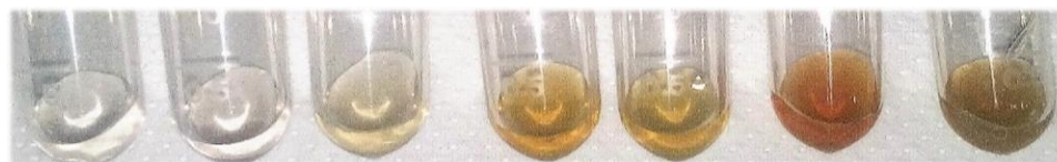
Figure 9- Colour differences of Au@Ag core-shell bimetallic NPs colloidal solutions obtained with different glucose concentrations in a range from 0 -to -1 mM (left to right).
