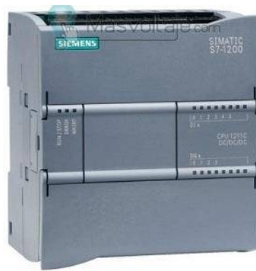
Figura 7. PLC SIEMENS S7-1200
