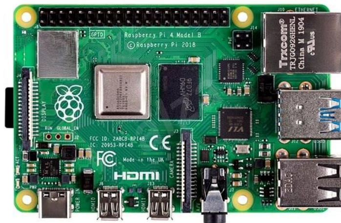
Figura 6. Raspberry Pi 4B. Elaborado por: (Raspberry Pi Foundation, 2018)
