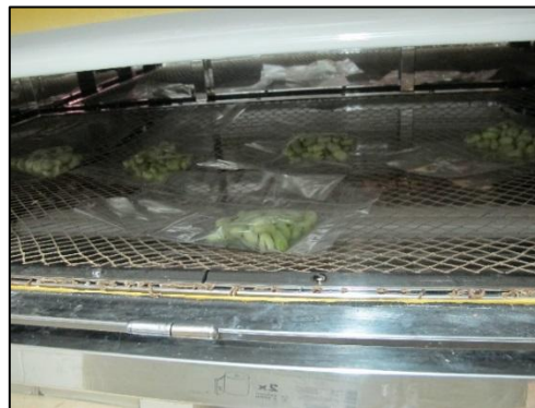
Figure 21. Faba beans sanitation with UV-C light at a pilot plant scale (discontinuous system).
