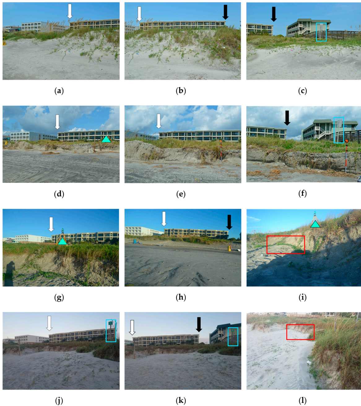
Figure 5. Site A field photographs showing conditions (a–c) pre- Irma , (d–f) post- Irma , (g–i) pre- Florence , and (j–l) post- Florence . Symbology denotes anthropogenic or natural locations that are consistent to more than one photograph.
