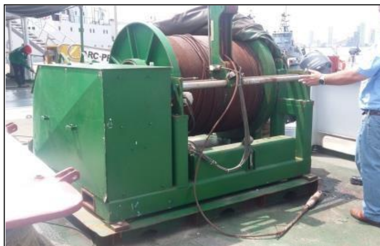
Figure 6. 2800 m geophysical research winch on board the ARC Providencia.
