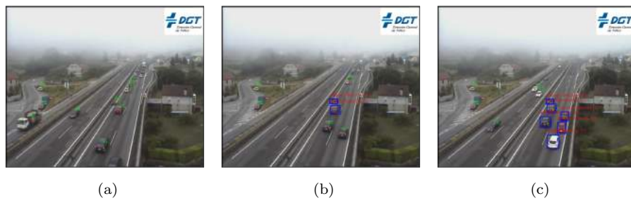
Figure 12: Example of an alarm for an accident. In (a) a motorcycle crashes with a car. In (b) the system detects both vehicles as static in a lane that has movement, so it triggers an alarm. Finally in (c) the system keeps triggering alarms for every car that stops in that area. Images courtesy of DGT.
