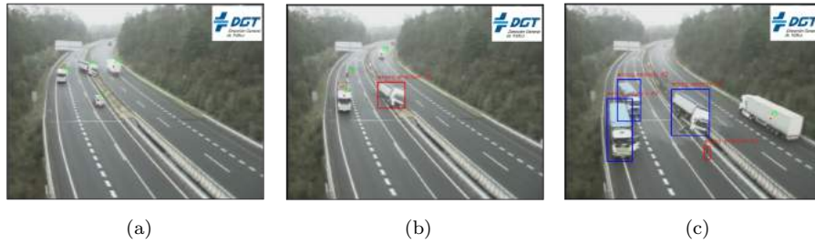
Figure 13: Frames of a video that has both alarms. In (a) a truck starts to derail. In (b) the system detects an anomaly in the second lane when the truck invades it so it triggers the wrong direction alarm. In (c) when the crashed truck remains static the system triggers the velocity alarm and it does the same for every truck that moves with abnormal velocity (reduced speed). Images courtesy of DGT.
