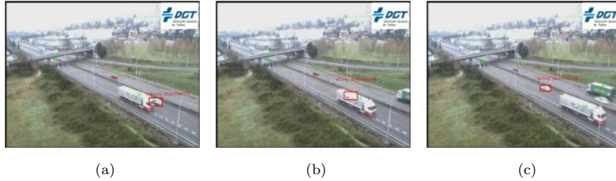
Figure 11: Example of an alarm for a vehicle moving in a wrong direction. In (a) the system detects an object moving with a direction contrary to the usual one in that lane, so an alarm is launched. In (b) the system keeps tracking the object despite being totally occluded. In (c) the system continues the tracking after the occlusion, keeping the same id and the alarm. Images courtesy of DGT.
