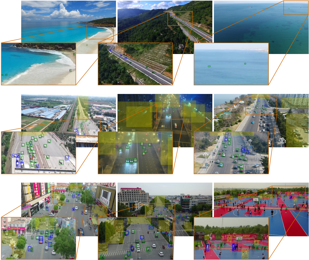
Figure 3.8: Some object detection results of STDnet-ST++ for USC-GRAD-STDdb (top), UAVDT (middle) and VisDrone2019-VID (bottom) test sets. A confidence threshold of 0.6 was used to display these images. For each image, green boxes are true positives, red boxes false positives and blue boxes false negatives. The yellow rectangles are ignored regions. Only objects that belong to the XS size are displayed.
