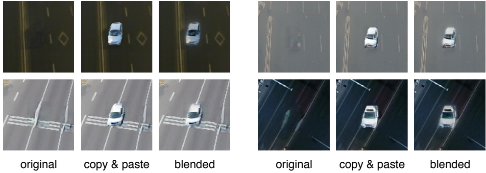
Figure 4.7: Image results of blending for similar synthetic small objects on different background conditions.
