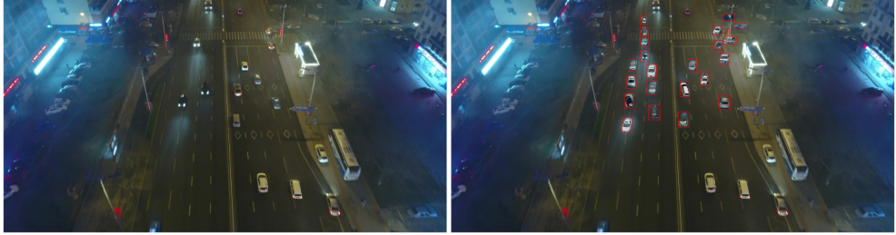
Figure 4.1: We describe a pipeline for small object data augmentation that is able to populate an original frame (left) with new generated small objects (right). New objects are highlighted with red bounding boxes.
