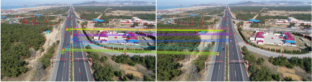
Figure 4.5: Motion angle estimation using optical flow for two frames f_i (right) and f_{i+1} (left). First, the feature points are computed using FAST (red dots). Second, f_{i+1} is stabilized with f_i by perspective transformation to remove camera motion. Then, the feature points are matched between frames (colored lines). Finally, the motion lines are summarized into a motion vector for each object (colored arrows).
