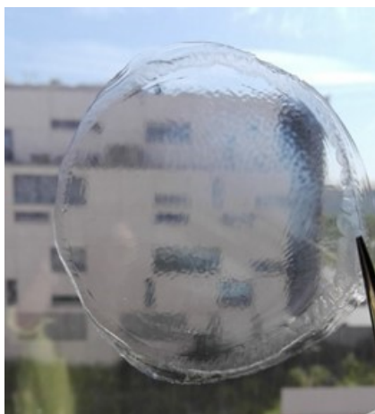
Fig. 1.9. PIM composed by PVC (base polymer) and D2EHPA (extractant).
