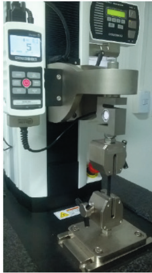
Figure 6. Tensile test set up. Source: Authors
