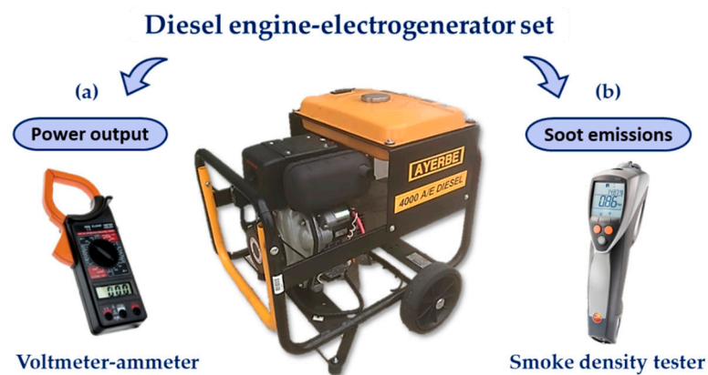
Figure 1. Scheme of experimental methodology to determine (a) power output by means of a voltmeter–ammeter device; (b) generated soot emissions by means of a smoke density tester, in a diesel engine–electrogenerator set [21].
