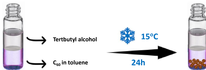
Figure 1. Schematics of the synthesis process for the C_{60} nanostructures
