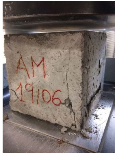
Figure 2. Compression strength test on cubic samples.
