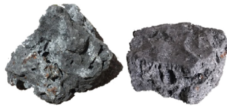
Figure 1. Electric arc furnace (EAF) steel slag used.
