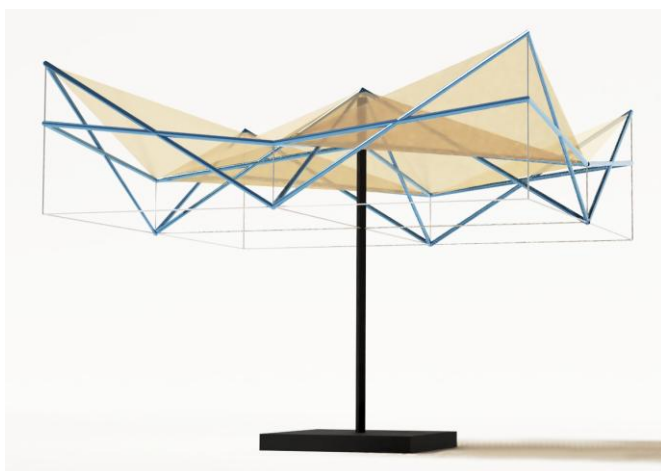
Figure 10. Expandable umbrella with square modulus
