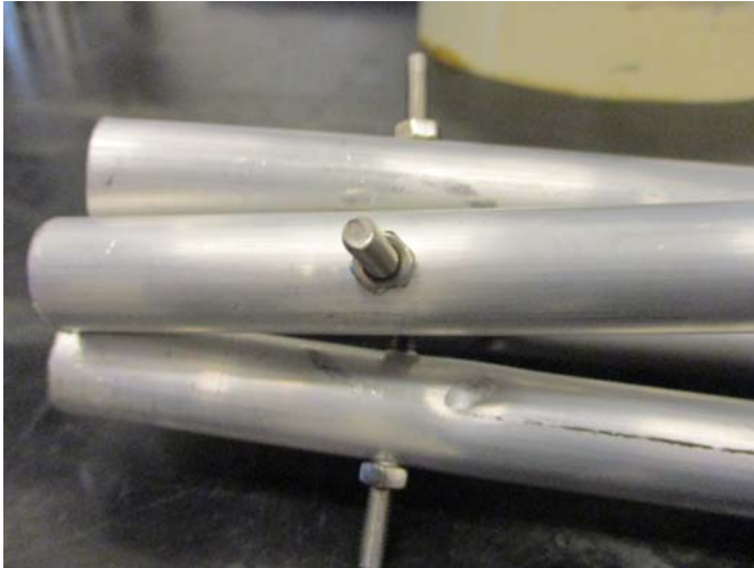
Figure 16.- Failure pattern for linkages with simple supported ends
