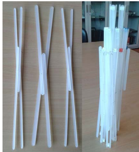
Figure 14: Folding of Compound Scissors, and Complete Folded Package Including these scissors.
