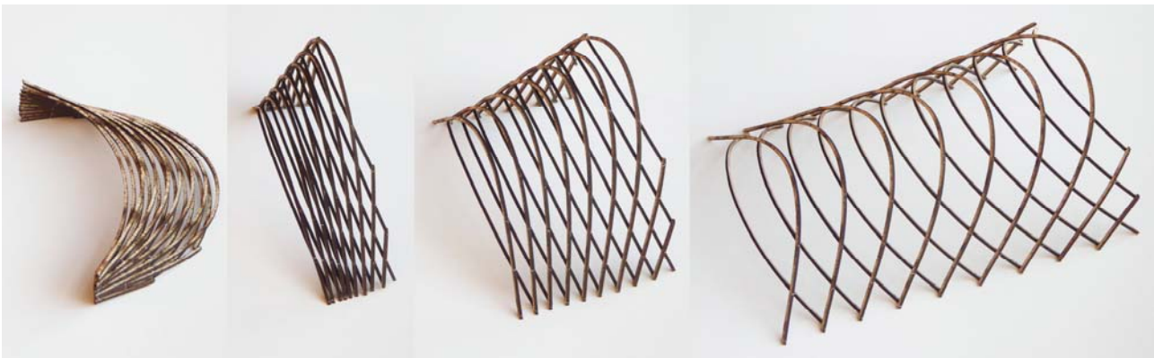
Figure 11: Deploying of the conoid vault
