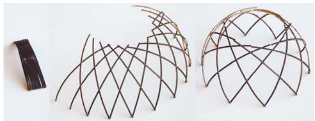
Figure 25: Deployment process of the concentric axes dome
