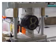
Figure 13. The tensile strength of the dry (ITSd) and the wet (ITSw) subset were then determined at 15°C.
