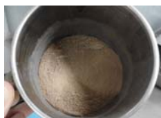
Figure 1. Waste cork dust as filler.
