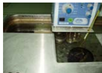
Figure 12. The "wet" subset was saturated and held in a water bath for 3 days at 40°C.
