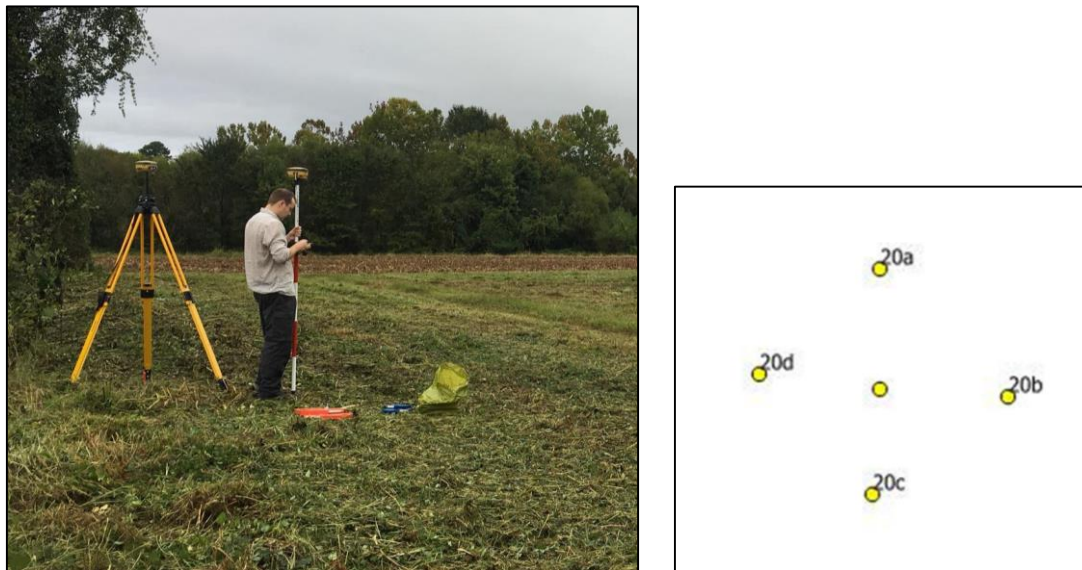
Figure 14: shows the author setting up the GNSS system (left) and the topsoil subsampling design for 1m 2 around the central sample location (right) (© author)
