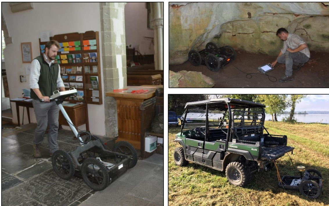
Figure 9: The versatility of GPR, A = surveying inside Deerhurst Church, UK, B = surveying cave sediments in Zanzibar, C = motorised survey in Virginia US (© M. Horton)
