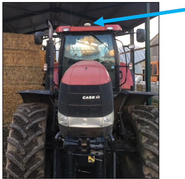
Figure 148: Topographical information from RTK GNSS points over the Wilsford henge (top) and example of tractor fitted with RTK GPS marked with blue arrow (bottom) (© author)
