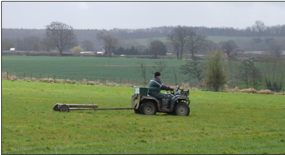
Figure 6: Precision Farming conductivity scan in progress (© author)
