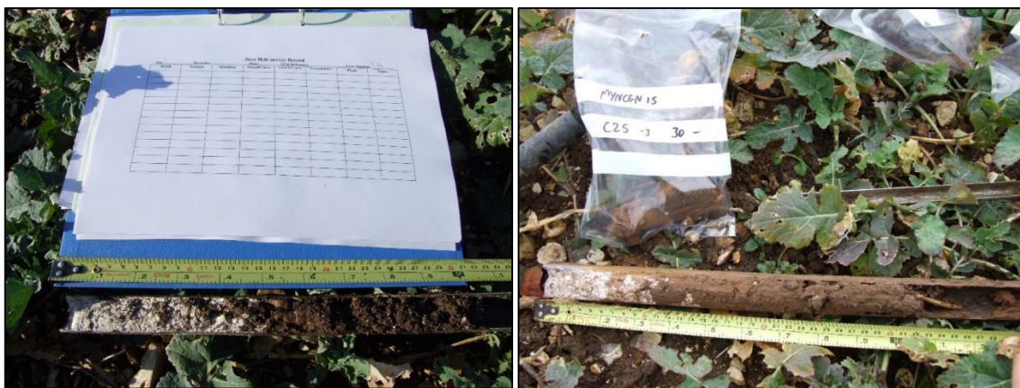
Figure 16: Gouge corer (25mm diameter) with a core (right) and the recording sheets used (left) (© author)
