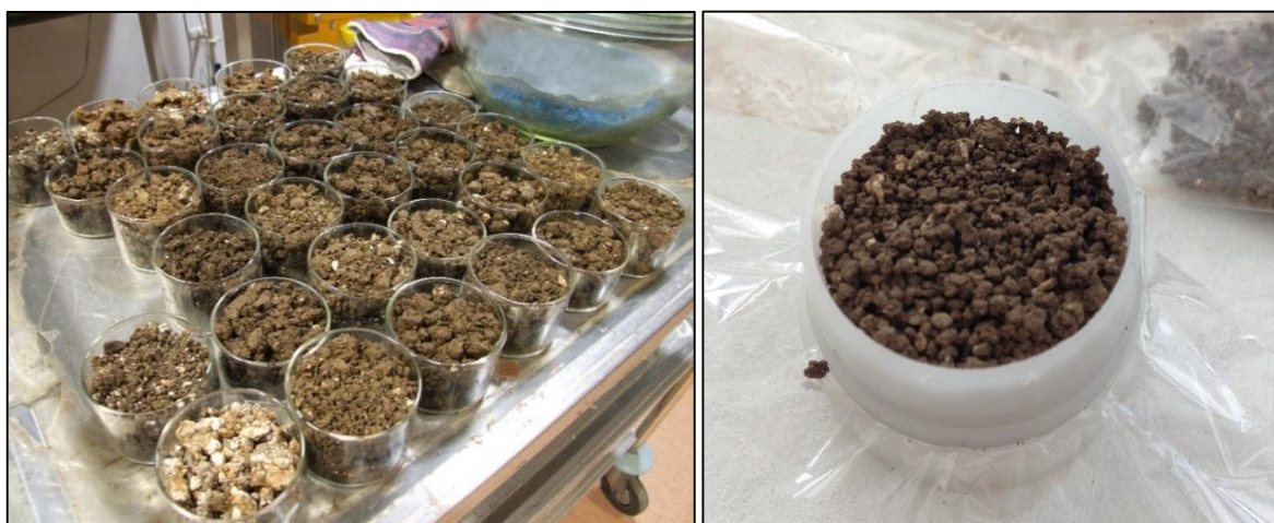
Figure 17: shows the 100g soil samples prepared for oven drying (left) and 10cl sample pot for pXRF analysis (right) (© author)
