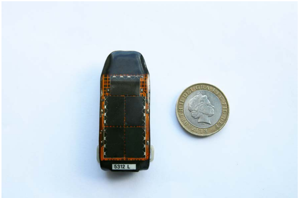
Figure 2.2: A GPS device from the University of Amsterdam Bird Tracking System (UvA-BiTS) used in this study with a £2 coin as reference. The GPS device is small (61x25x10 mm), lightweight (~13.5 gram), solar-powered with rechargeable batteries, has an internal antenna and high memory capacity (~220 mAh).
