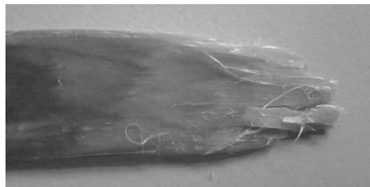
Figure 2-13 Digital image of extruded pea protein isolate of 55% moisture content at a cooking temperature of 160°C, exhibiting predominant lengthwise fibrous structures. Reproduced with permission from Elsevier; Osen et al. (2014).
