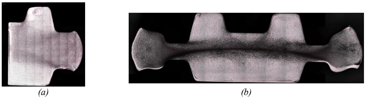
Figure 4. Macrographs of IN718 forged on a screw press at 970°C: (a) half-forged (one half of the cross-section) and (b) fully forged part.
