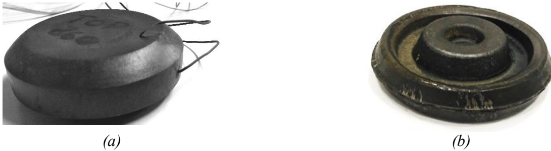
Figure 3. Representation of geometry used in the present study: (a) double-truncated cone; (b) profiled disk
