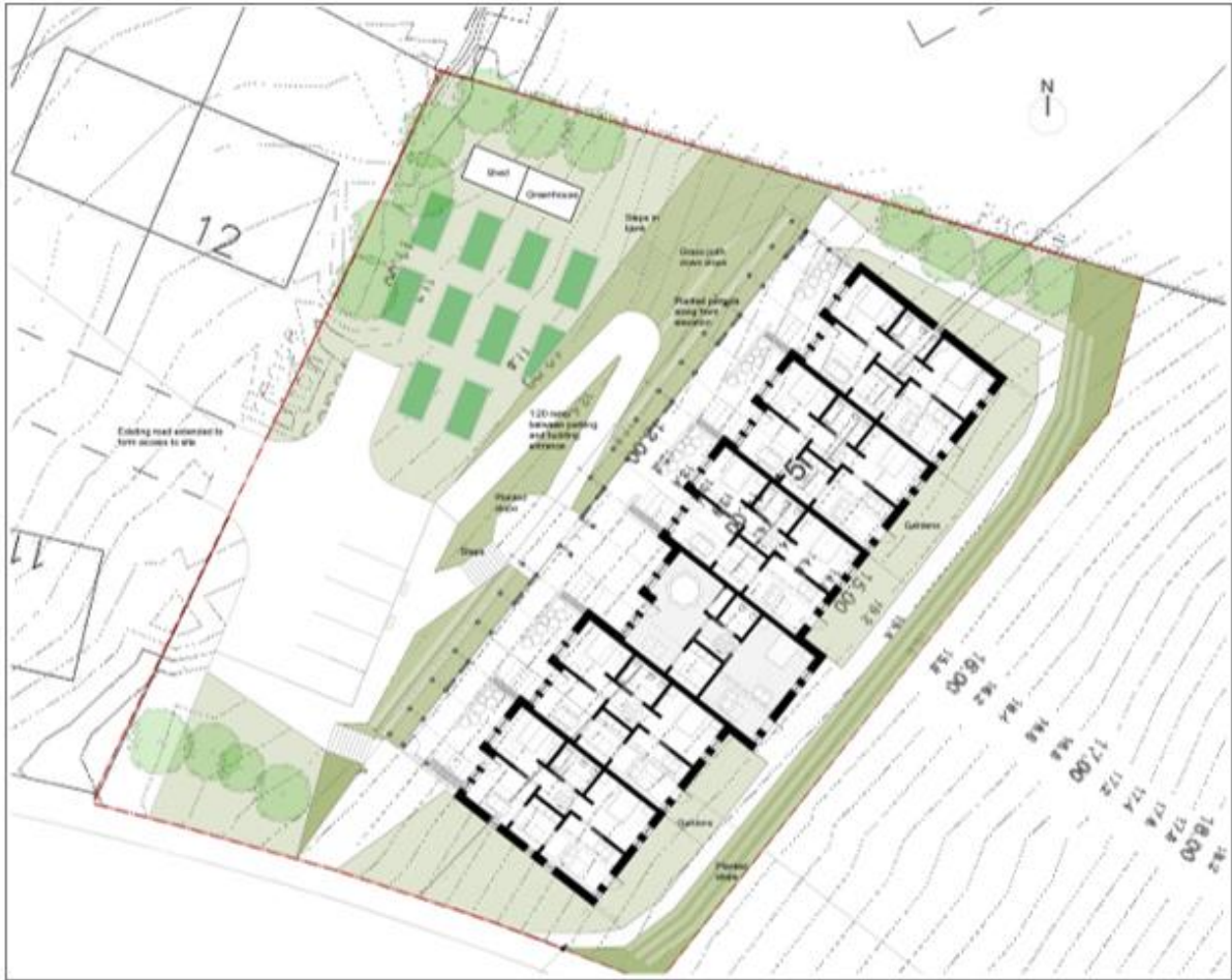
Figure 1: Proposed site plan showing the access from Taftingus Place (to the left), communal and private garden areas, and arrangement of individual houses and social corridor
