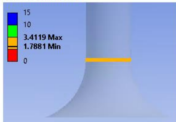
(c) Fatigue safety factor for maximum stress in shaft
