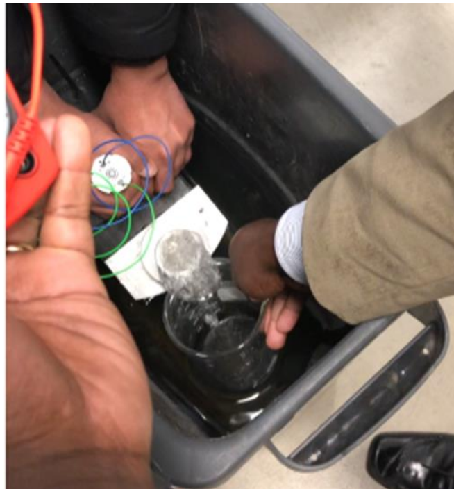
Figure B.5: Mechanism and water pumping test of 3D printed concept pump model.
