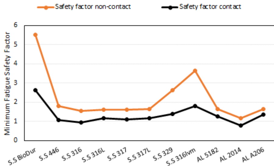
Figure 5.17: Minimum fatigue safety factors comparison of piston shaft assembly with and without contact region with optimised slider diameter with selected materials.
