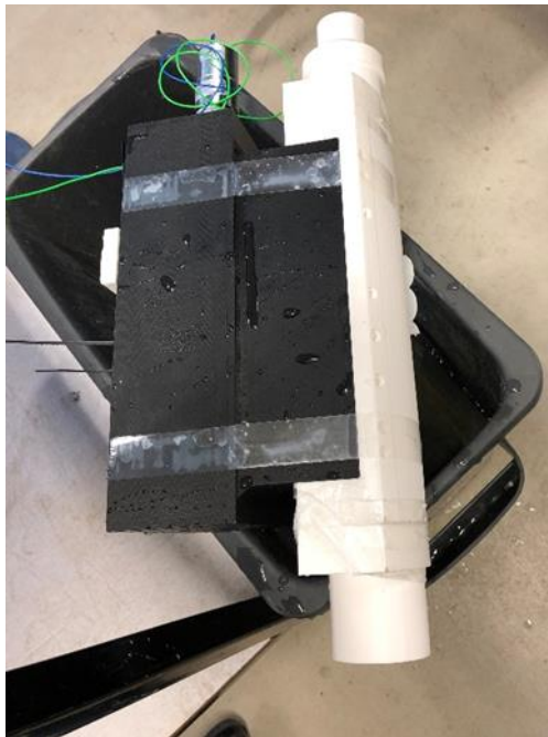
Figure B.4: An illustration of printed pump parts assembly.
