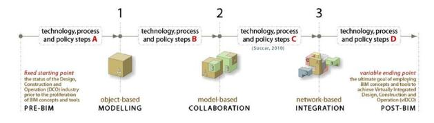
Figure 2.4: Step sets leading to BIM Stages (Succar et al. 2013)
