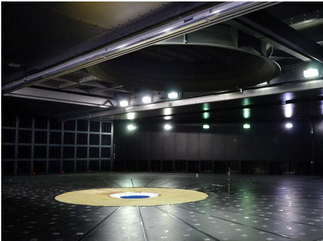
Figure 3-1: WindEEE Dome chamber showing the 60-fan wall and bell mouth (Hangan et al., 2017)
