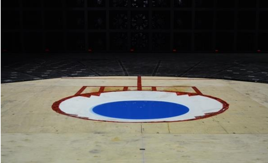
Figure 3-4: Water tank installed flush with chamber floor in WindEEE testing dome
