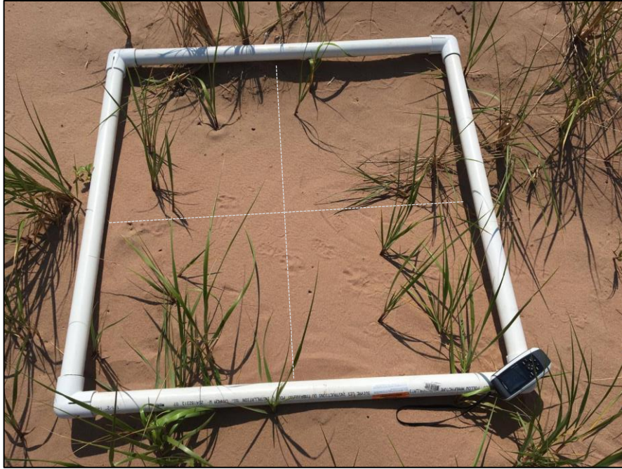
Figure 11. Delineated area for vegetation and soil sampling. Visual quadrants were used as a guide for representative sampling.
