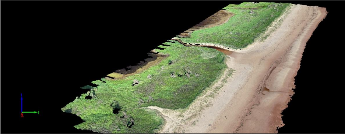
Figure 43. High density point cloud of the inlet found in Stanhope beach at profiles 6290m – 6320m.
