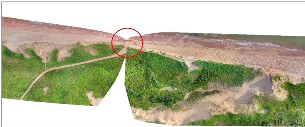
Figure 34. 1.4cm/px resolution orthomosaics showing the location along Brackley beach, profile ~3920m, where a ramp connecting the beach to an access point decreases the beach width.
