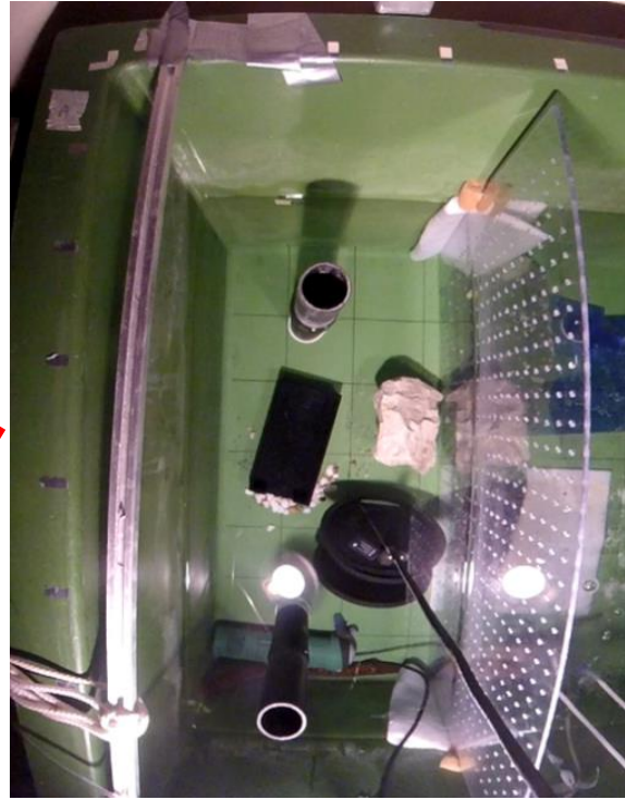
Figure 3.1. Side view and top-down view of experimental setup. A) The red oval indicates the camera attachment where the camera would have a birds-eye view of the tank. The red circle indicates the speaker set up in the middle of the tank. The red square shows the battery and amp that are attached to the speaker to provide the power and the arrow points to the lamp that provides the light so that the camera can pick up movement. B) An example frame of the view from the experiment camera.
