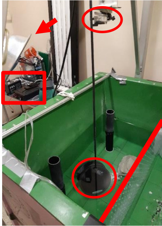
Figure 3.1. Side view and top-down view of experimental setup. A) The red oval indicates the camera attachment where the camera would have a birds-eye view of the tank. The red circle indicates the speaker set up in the middle of the tank. The red square shows the battery and amp that are attached to the speaker to provide the power and the arrow points to the lamp that provides the light so that the camera can pick up movement. B) An example frame of the view from the experiment camera.
