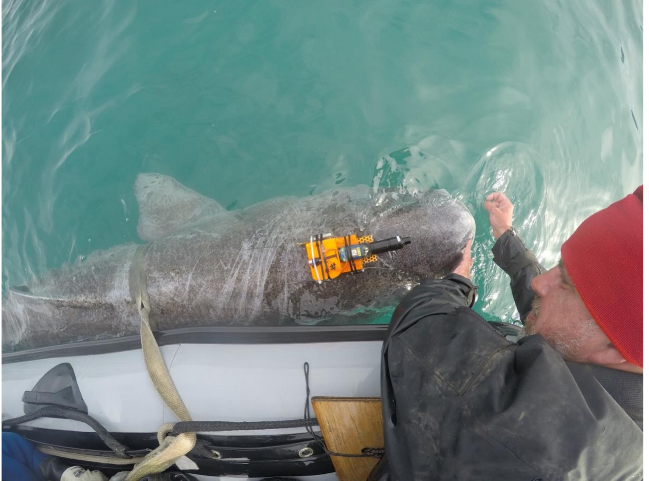
Figure 3.1: Photo depicting the placement of a biologger package on the superior dorsal region of a shark.
