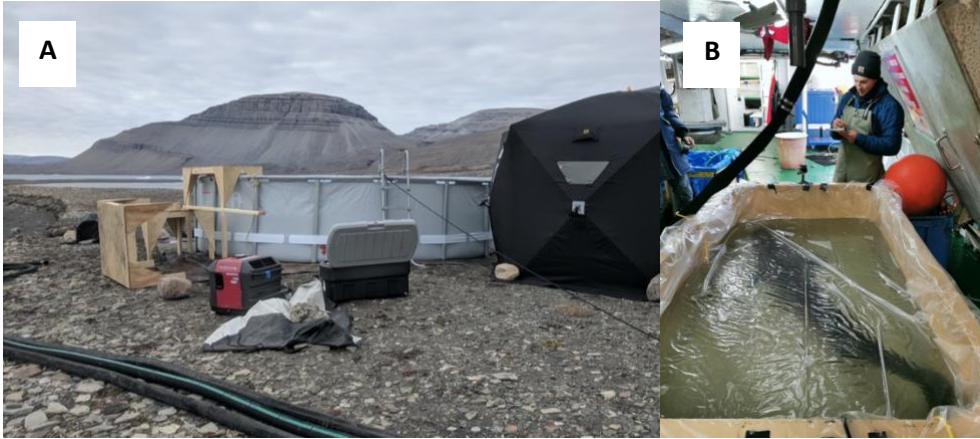
Figure 2.2: Photographs of the two respirometers used in this study. Panel A depicts the large “circular” type respirometer used in Tremblay Sound in 2018 (Photo by Eric Ste-Marie). Panel B depicts the smaller “rectangular” type respirometer used in Scott Inlet in 2019 (Photo of E. Ste-Marie taken by Jena Edwards and used with permission).
