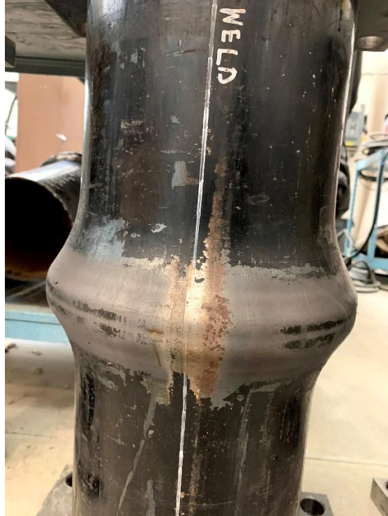
Figure 4.29: Visible Flat Appearance at Wrinkle Crest for Specimen IP60WA10.5
