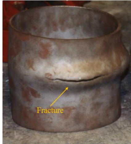
Figure 1.1: Fractured Field Pipeline of Wascana Energy Inc. (Courtesy of Wascana Energy Inc.)
