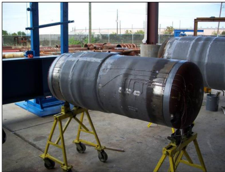
Figure 2.15: Picture of the Specimen Showing Strain Gauges and Repair Location (Alexander and Kulkarni 2009)
