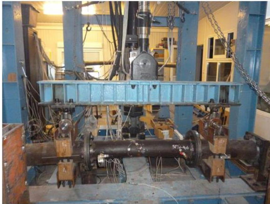
Figure 2.22: Monotonic and Cyclic Bending Setup for Dented Pipe Specimen (Pournara et al., 2015)
