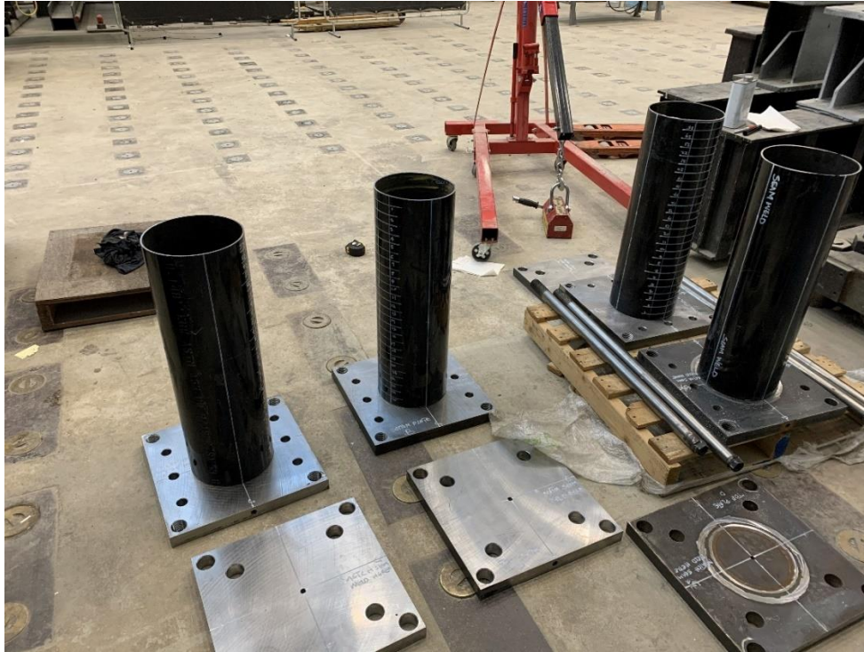
Figure 3.3: Cut Pipe Specimens with Appropriate Markings and Straight Bars
