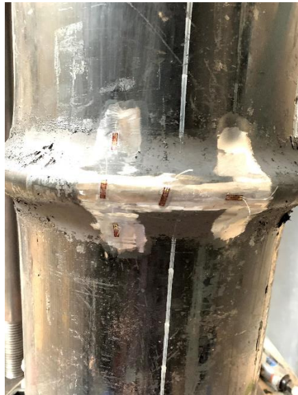
Figure 3.16a: Strain Gauge Configuration on Wrinkled Pipe.
