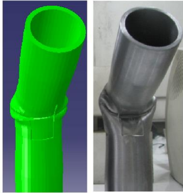
Figure 2.7: Collapsed Form of a Defected Specimen Subjected to Cyclic Axial Loads (Zeinoddini et al., 2015)
