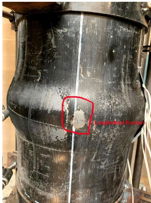
Figure 4.30: Visible Longitudinal Fracture at Wrinkle Crest for Specimen IP60WA6
