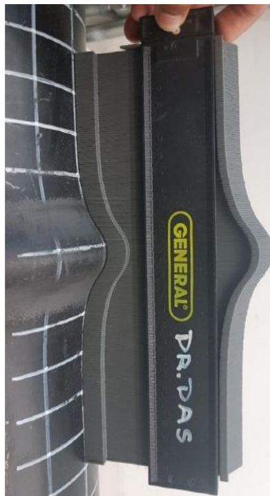
Figure 3.11: Wrinkle Profile Measurement using Contour Gauge
