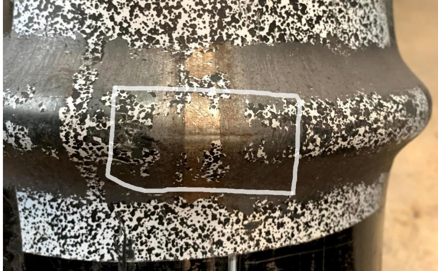
Figure 4.19: Visible Circumferential Fracture at Wrinkle Crest for Specimen IP30WA8
