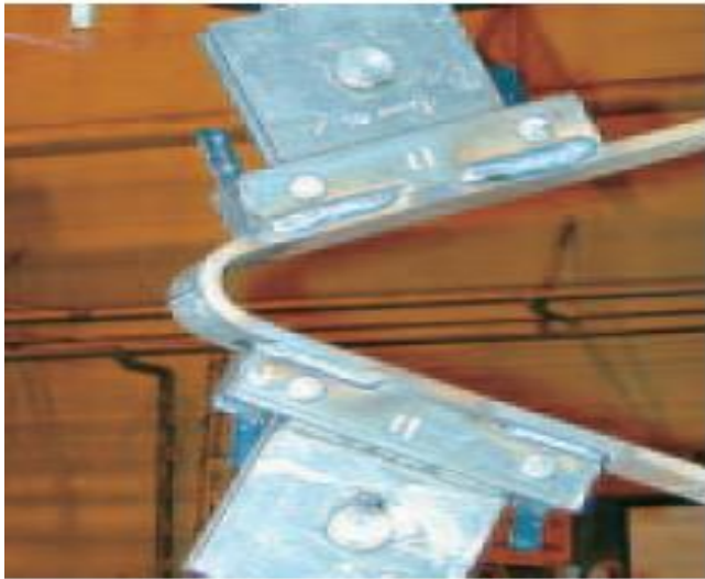
Figure 2.24: Strip Specimens Cut from Pipes (Das et al., 2007b)
