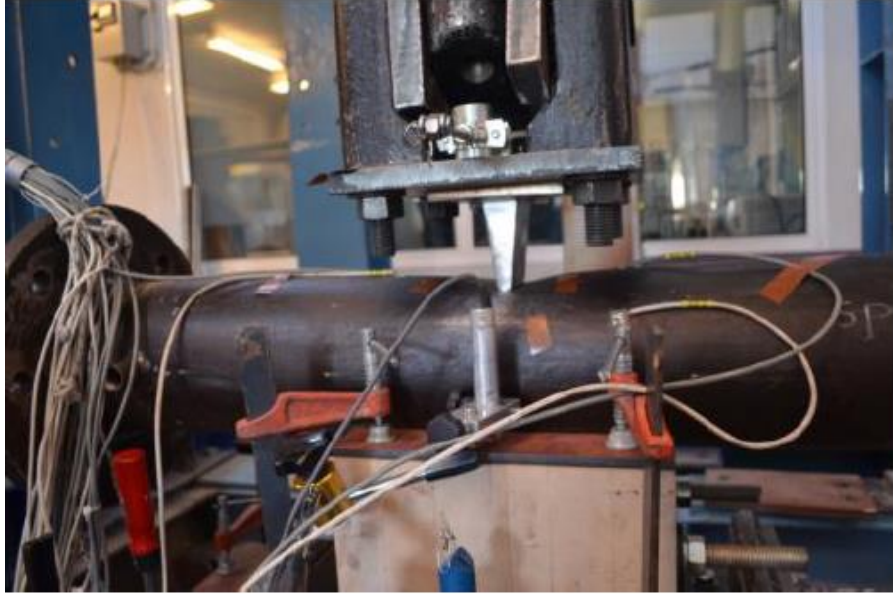
Figure 2.21: Denting Setup for Pipe Specimen (Pournara et al., 2015)
