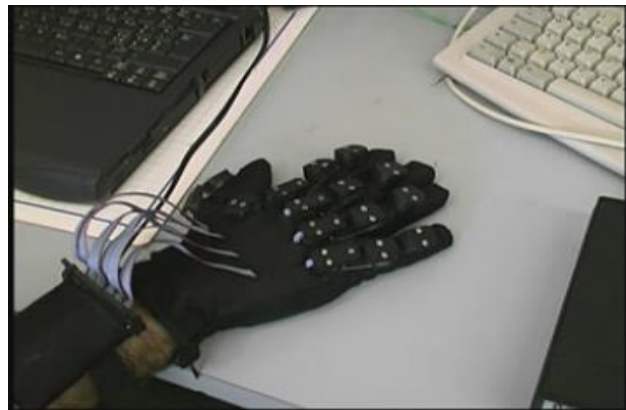
Figure 4 An Example of a Hall-effect Based Sensor Glove [55]
