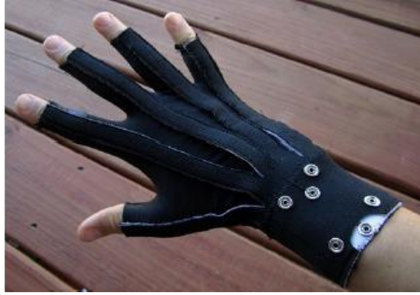
Figure 5 An Example of a Flex Sensor Based Glove [55]
