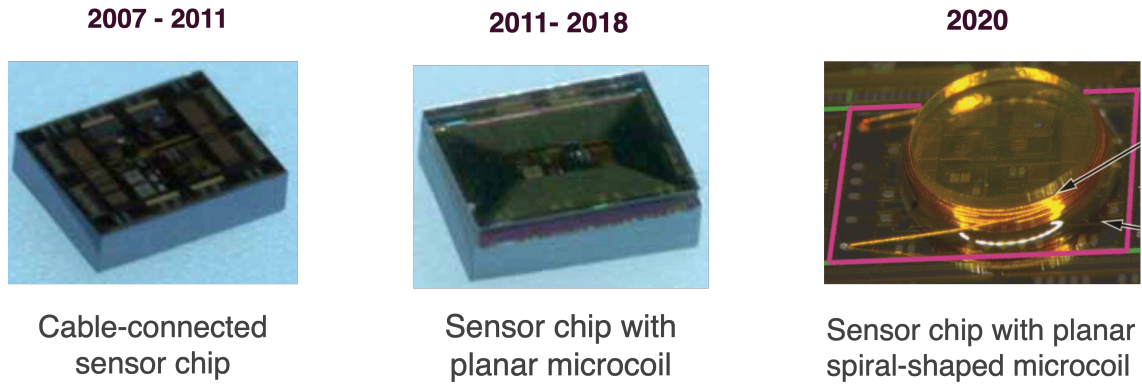
Fig. 2 : Evolution of chip (macrograph)
