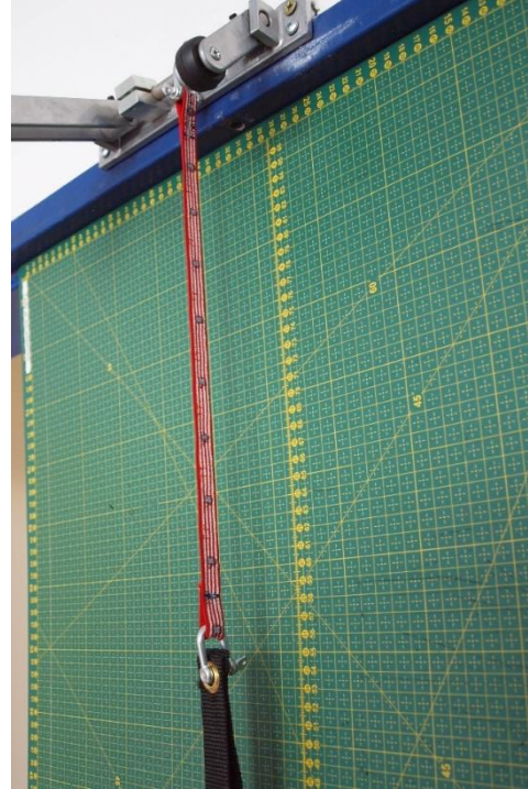
Fig. 4: The ribbon during jerk test in relaxed length
