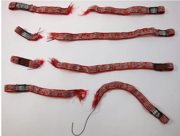
Fig. 6: Tested ribbons after the jerk test.
