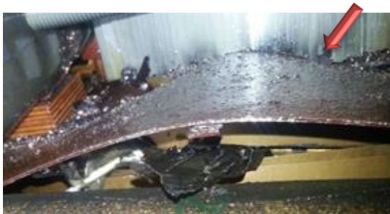
Fig. 7: Exposed damaged winding of the transformer HV coil. The short circuit is located about 50 degrees from the busbar. The combustion plant has an irregular shape and a range from the surface to the first cooling channel.
