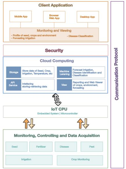
Figure 2 Mapping agriculture taxonomy with IoT architecture stack
