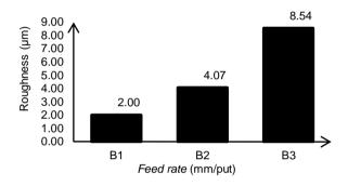
Figure 10. Response to surface roughness level feed rate
