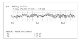
Figure 12. Smoothest condition surface roughness graph
