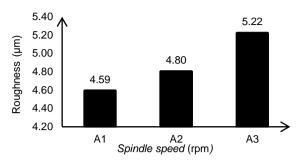
Figure 9. Response to surface roughness level spindle speed
