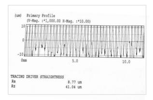
Figure 14. Roughest surface roughness graph.
