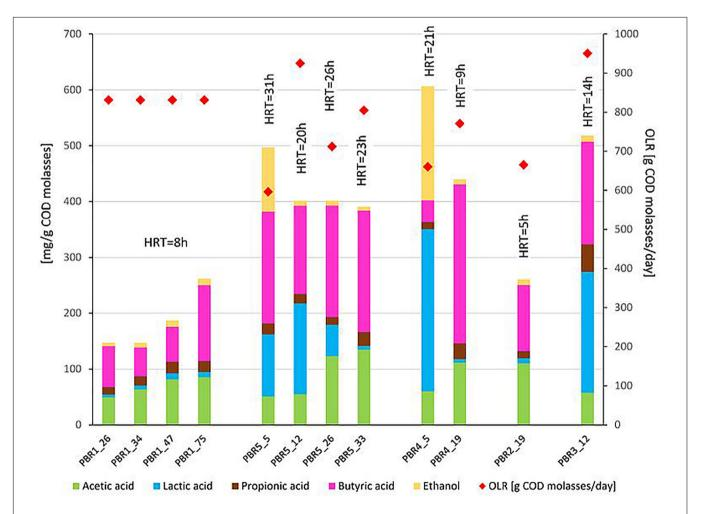
FIGURE 2 | Non-gaseous fermentation products expressed in mg per g of COD of molasses (bars, left axis) and substrate concentration in g of COD of molasses per day (diamonds, right axis) supplied to the bioreactors in selected time points of operation. The composition of fermentation products was analyzed using high-performance liquid chromatography. The data comes from two parallel measurements. HRT is shown over each bar.
