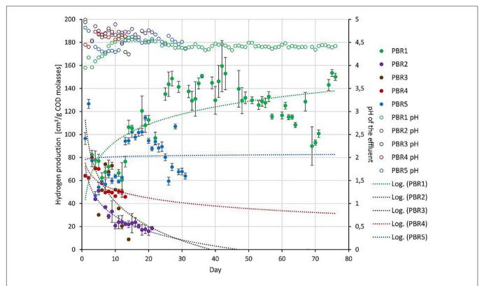
FIGURE 1 | The long-term performance of PBRs tested in this study: hydrogen production (solid circles, left axis) and pH of the effluents (open circles, right axis) from bioreactors. Since the operation periods were different, trend lines were added for hydrogen-production data sets.
