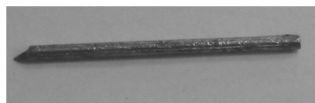
Fig. 50. An example of a sample obtained by the vacuum suction casting apparatus
