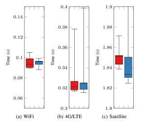
Fig. 5. MQTT performance over TCP and QUIC: time required to publish a message after connection establishment. Red Whiskers is for QUIC and Blue ones is for TCP
