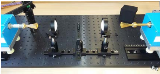
Fig. 16. W-Band quasioptical system with 4f topology ( f = 75 \text{ mm} ). Mm-wave Extension modules V10VNA2 WR-10 (OML), horn antennas and PTFE lenses.
