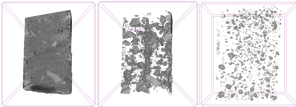
Fig. 7. RAC2 specimen (left), coarse LA in it (center) and its closed porosity (right).
