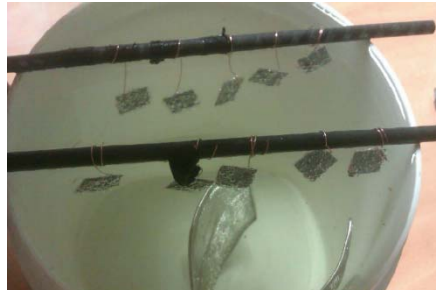
Figure 7. SPT pre-embrittled specimens during its hydrogen absorption.
